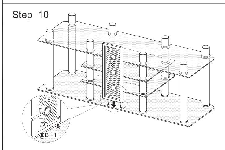
To attach cable management system (8) to the stand, place appropriate holes of cable management system (8) over short rods (B). Screw cap nuts (C) onto short rods (B) and tighten with wrench (F).
